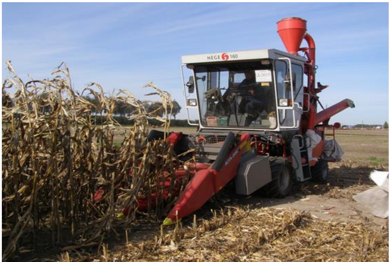
Pic.4. Small-sized combine harvester "Hege 160" with a modular system for replacing the header from the grain type to the corn type, "Octyabr variety testing station"
