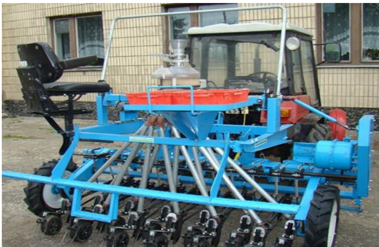
Pic.2. Small-sized seeder for sowing grain, leguminous and other agricultural plants "Wintersteiger TRM" (Austria), Kobrin testing station
