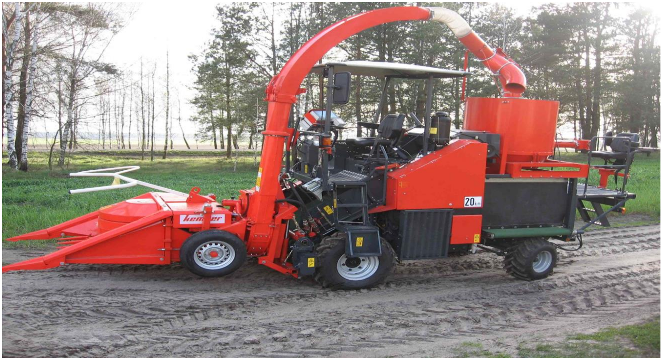
Pic.3. Small-sized fodder harvester combine «Sibus» («Hege212») with electronic balance for harvesting of forage herbs and maize for silage, Mozyr testing station.
